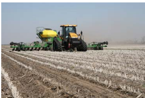
Figure 2. No-till drill application of polymer to field
